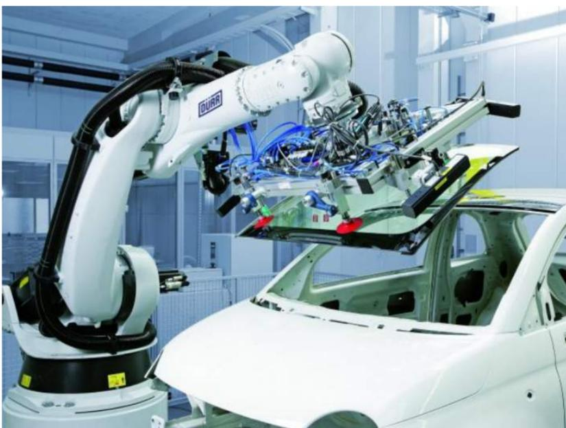
Any semblance that it bears is to a severed, independent human arm, which is exactly what it has been designed to replicate in function. Such factory robots can lift and assemble heavy machinery, weld pieces of metal together, and even tighten screws just like a human hand.
